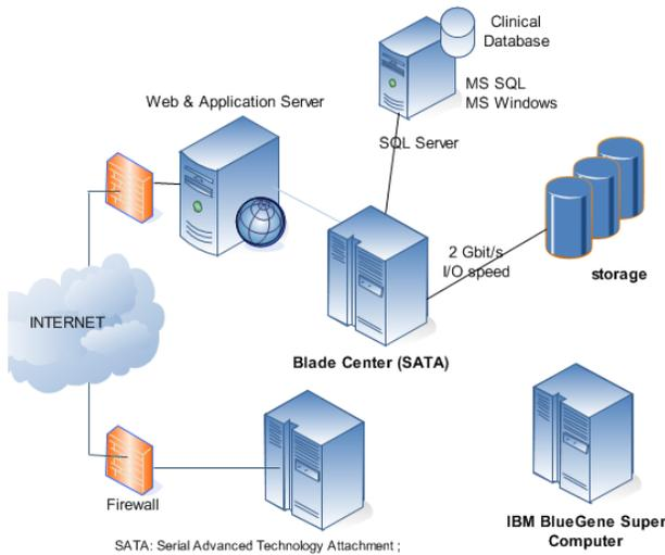
Fig. 1. Information technology structure for the THEW. Two options are proposed to access the data from the THEW: 1) Server hosted at University of Buffalo based using secured file transfer protocol (SFTP) , 2) THEW client application which is a dotNET client server application providing the access to both ECG signals and the associated clinical information
